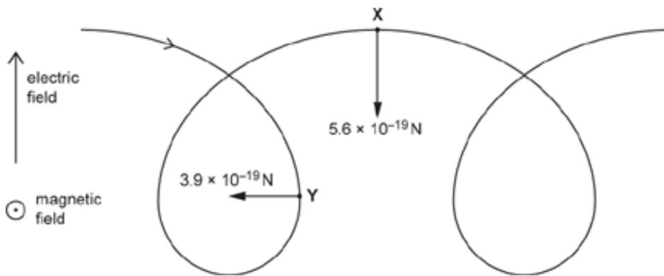
The uniform electric field is directed upwards, with electric field strength  $E = 0.90 \text{ N C}^{-1}$ .
